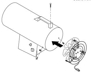
Figure 13 - Replacing Motor and Fan Guard into Heater
